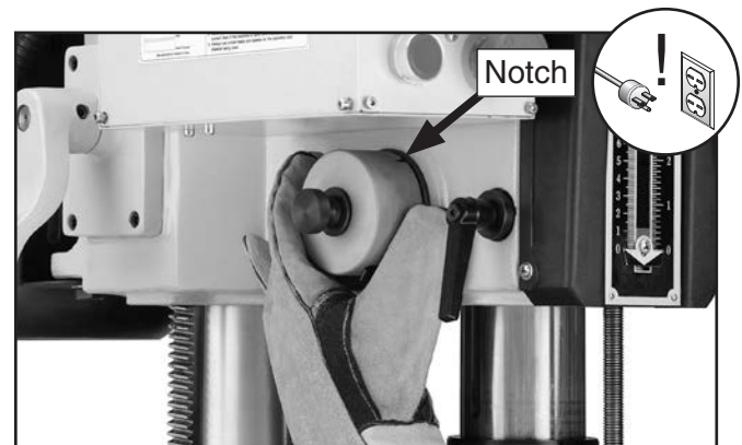
Figure 45. Example of adjusting spring tension by rotating spring cover to engage next notch with roll pin.
